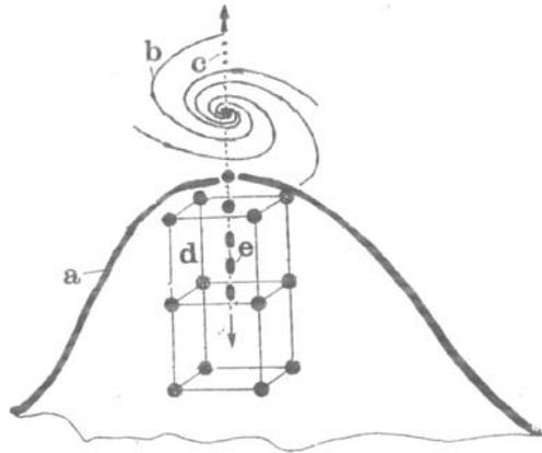
**Figure 1.** Schematic presentation of a micropinch spiral by tip effect in the electrolysis cell: a) tip of the electrode; b) spiral structure of micropinch; c) electron beam; d) crystal channel; e) ion beam.
